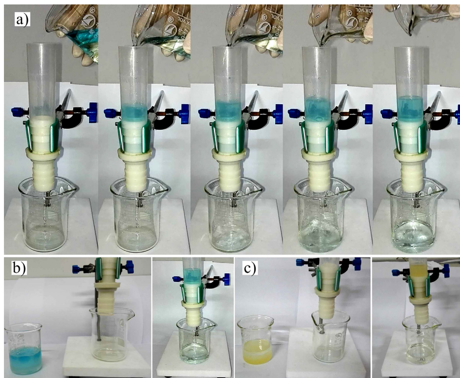
Fig. 8. Oil-water separation process by using the \text{TiO}_2 modified copper mesh (microstructure space of 0.10 mm): (a) separation process of trichloromethane-water emulsion, (b) photos of trichloromethane-water emulsion before and after separation, (c) photos of cyclohexane -water emulsion before and after separation.
